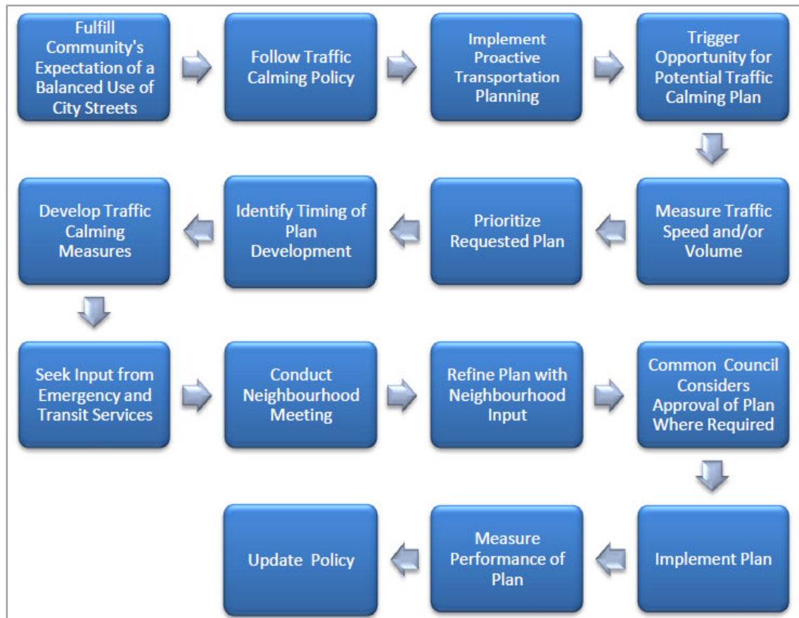
Exhibit 2-1: Traffic Calming Plan Implementation Process (Source: City of Saint John Traffic Calming Policy)
