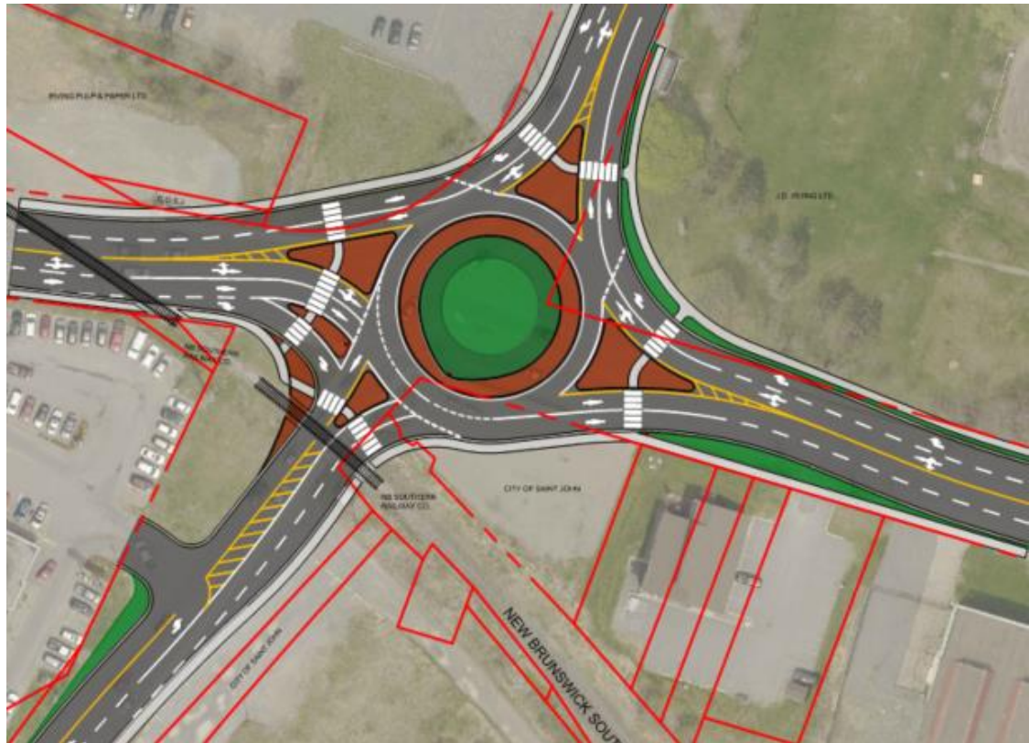
Exhibit 3.7: Simms Corner Roundabout Multi-Lane Roundabout Concept
