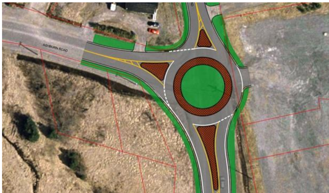
Exhibit 3.3: Rothesay Road/Ashburn Road Single Lane Roundabout
