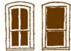
No: Arched top has been removed. Vertical muntin bars have been removed. Original style and proportions have been lost.
